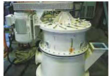
SCIROCCO head for Pendular Roller Mill
