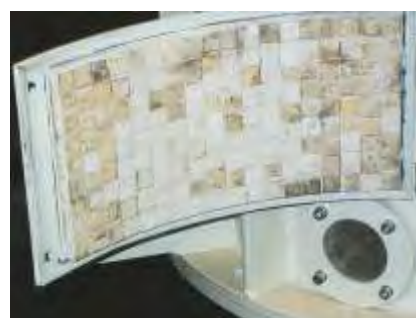
SCIROCCO with internal ceramic lining
