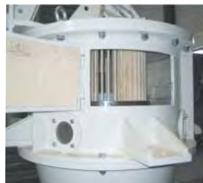
SCIROCCO 200CD for abrasive products with ceramic flaps
